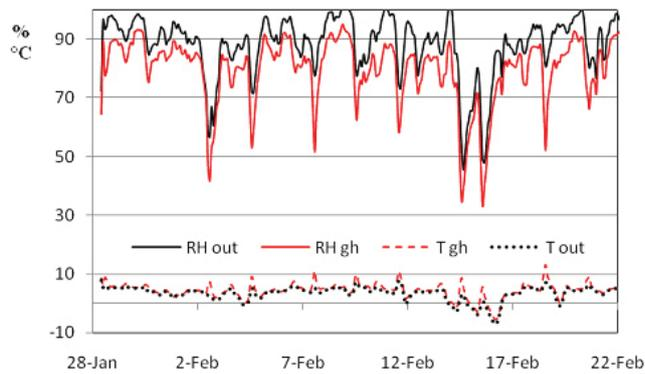
The graph below shows logged temperature in February for the Glass House respectively outdoor temperatures. When the sun appears the temperature reaches 15 C.
