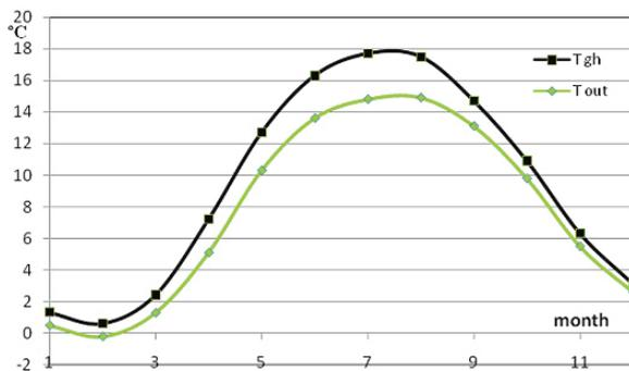
A theoretical simulation of the temperature in the Glass House for this project in relation to expected outdoor temperatures.
